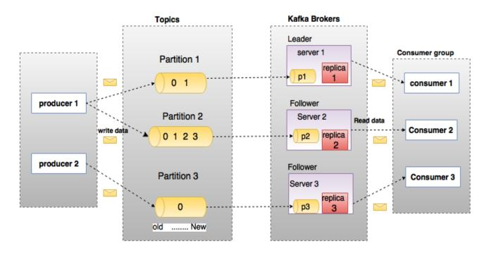
In the above diagram, a topic is configured into three partitions. Partition 1 has two offset factors 0 and 1. Partition 2 has four offset factors 0, 1, 2, and 3. Partition 3 has one offset factor 0. The id of the replica is same as the id of the server that hosts it.
