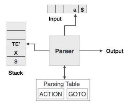
Predictive parsing uses a stack and a parsing table to parse the input and generate a parse tree. Both the stack and the input contains an end symbol **\$** to denote that the stack is empty and the input is consumed. The parser refers to the parsing table to take any decision on the input and stack element combination.
