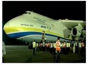
maximum speed is 850 km per hour with a 15,400 km range and 11,000 meters cruising altitude.
