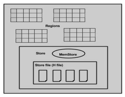
The store contains memory store and HFiles. Memstore is just like a cache memory. Anything that is entered into the HBase is stored here initially. Later, the data is transferred and saved in Hfiles as blocks and the memstore is flushed.
